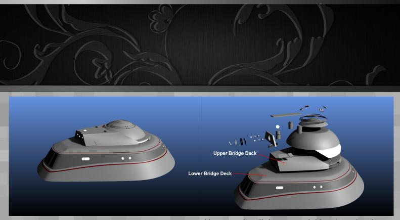
The bridge assembly consists primarily of two tear drop shaped objects and two partial spheres. The two teardrop meshes were built using smoothed vertex objects. Windows were mapped using a top down projection along with the top red line detail. However, texture mapping the red line along the bottom was very difficult to achieve with a good result. Therefore, more vertices were added and an additional shading domain was put in to add the lower red line.
